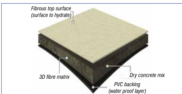
Figure 8 – Components of Geosynthetic Gliddenous Composite Mat
