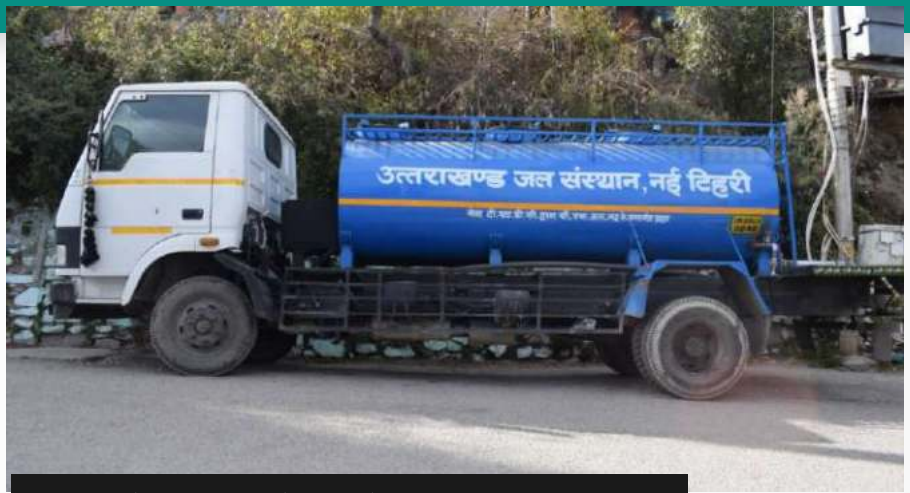
Mounted Water Tanker with 5,000 liters capacity
